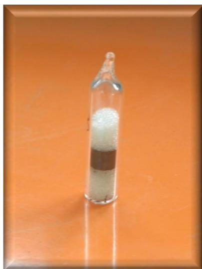
Encapsulation MAX phases samples
