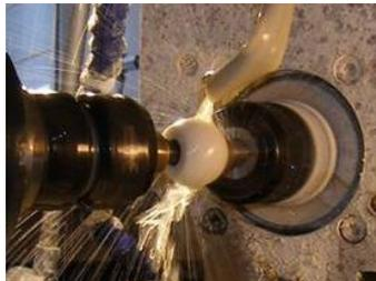
Making of ball head from nanostructural zirconium dioxide
