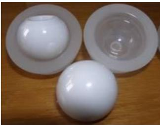
Bearing pair 'sapphire/nanostructural zirconium dioxide' for total hip-joint prostheses
